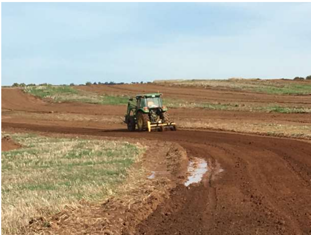
Figure 6. Tractor with Power Rake conditioning the soil
